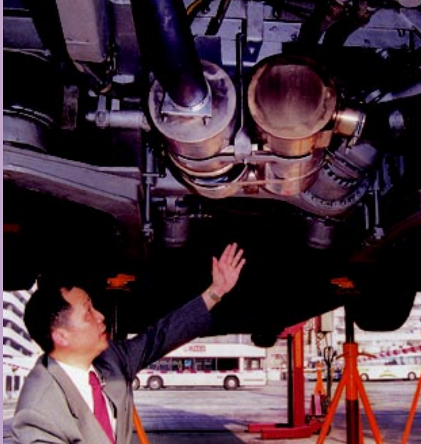
KMB's Engineering Manager introduces the catalytic converters, which will be installed on all pre-Euro I engine buses during 2000
