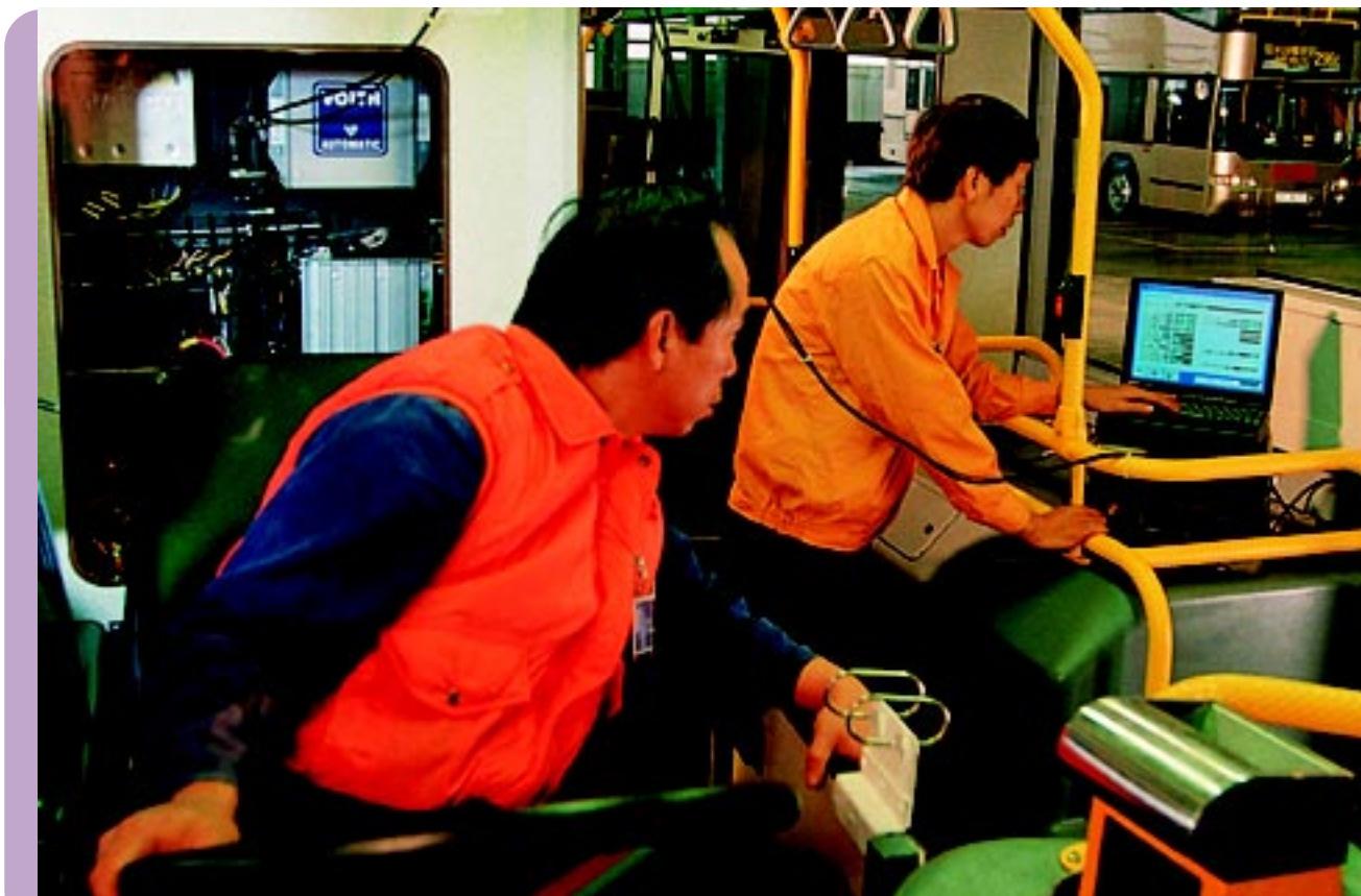
Computerised diagnosis of buses in all depots ensures high degree of mechanical reliability
