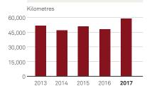
Average number of kilometres operated before one mechanical breakdown while passengers are on board
