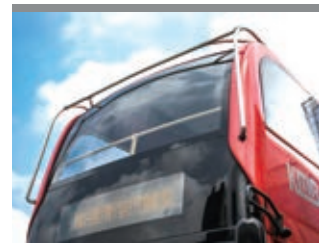
More tree guards will be installed to protect the bus windscreen and body from branches and twigs
