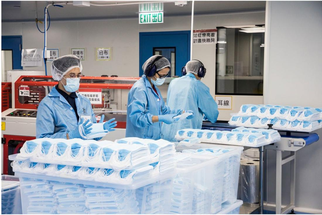
All self-produced face masks are locally manufactured and the cleanliness of the clean room meets ISO class 8 under ISO 14644-1 and has obtained the certification of ATSM Level 1.
