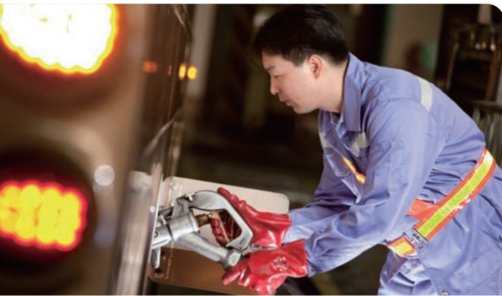
The aircraft-style "Posilock" fuel filling system as used on KMB buses
